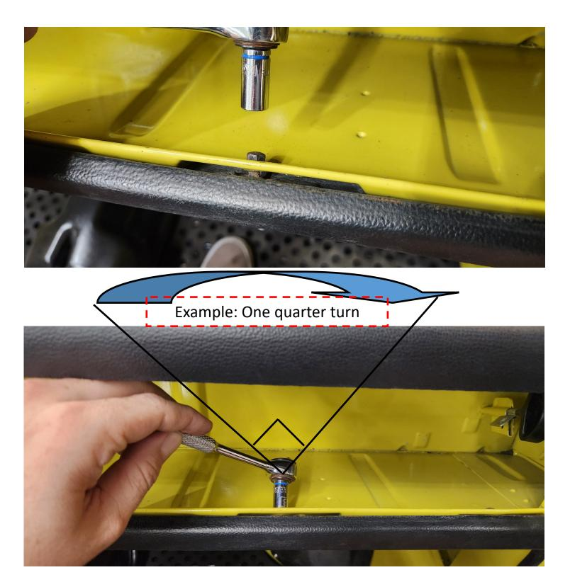
Note: There should now be a small gap between the glove box lip and the padded strip. This gap will be where the hinge tabs will be sandwiched together.
