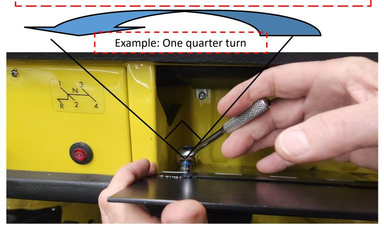
5. Find the location of the glove box lock which is directly above the latch, then with the tool provided, slightly bend the inside lip out until the glove box door latches.
