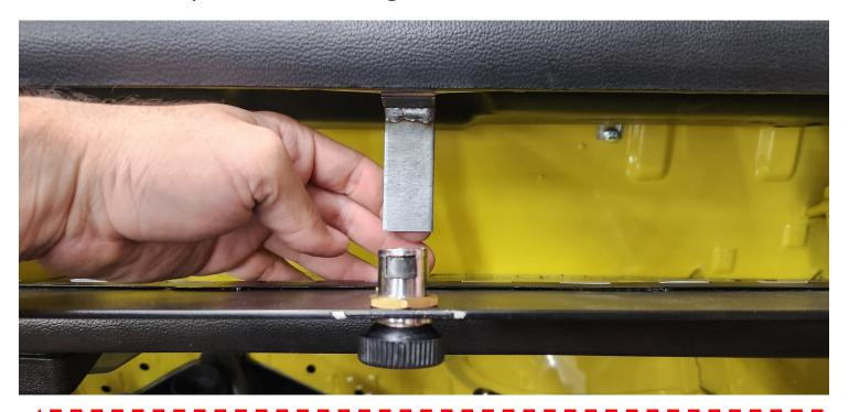
The metal should only be slightly bent out to reach the latch. It is recommended to only bend little by little until the glove box lock latches.
