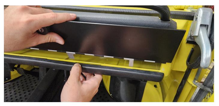
3. Lower the door so that the hinges are slightly above the padded strip.
