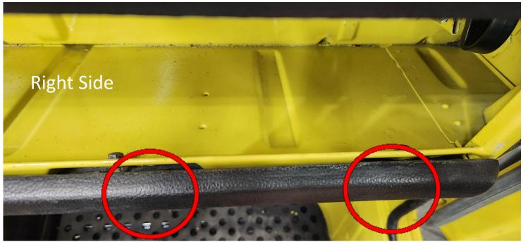
2. The padded strip should now be loose. Next insert each of the hinge tabs between the dash and the padded strip. Be careful to align glove box door with the edges of the glove box.
