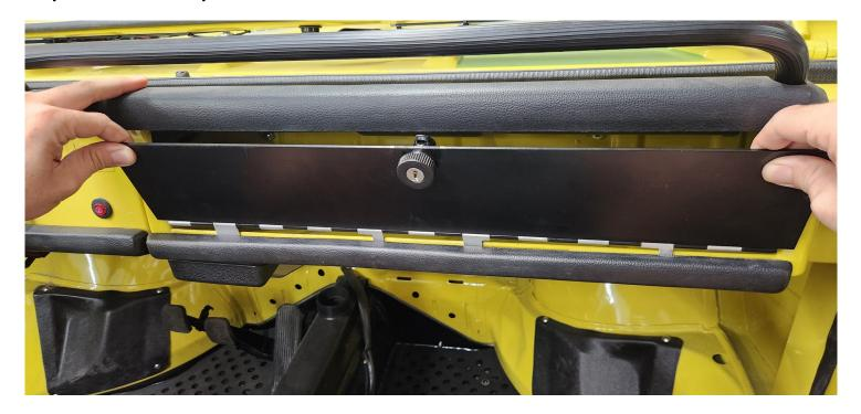
4. Tighten 4 nuts 4-6 quarter turns or as necessary.
